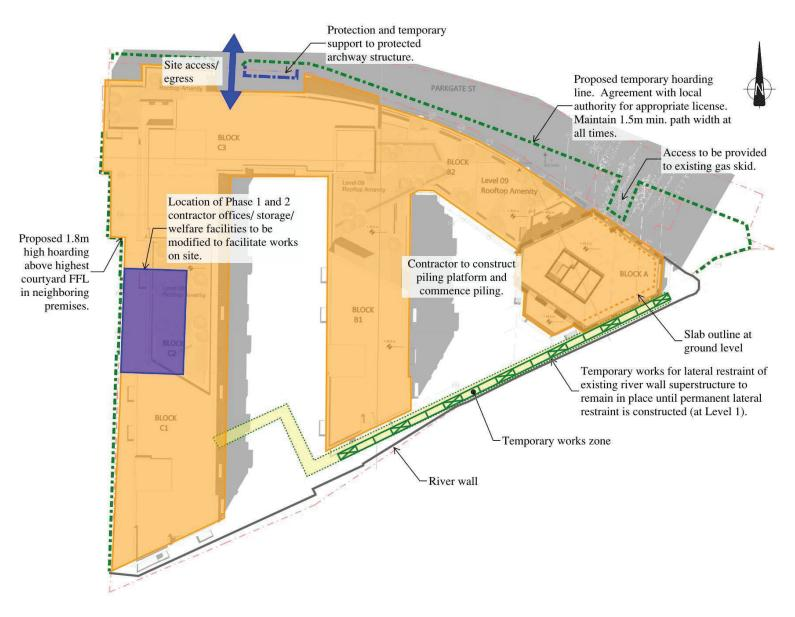
Figure 2: Overall sequencing of Works (2 of 6)
