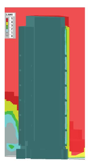
Figure 2.4.2 - Balcony Comfort - Section Through Tower Balconies from South East
