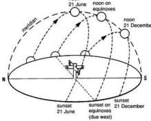
Fig 2.1.1 -Sample Sunlight Image & Sun Path Diagram
