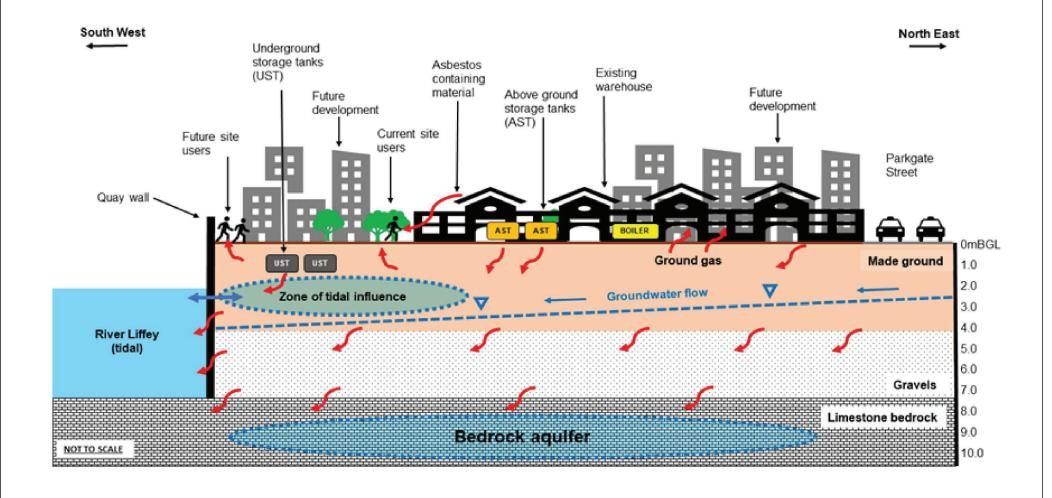
The Preliminary Conceptual site model is updated based on the findings of the ground investigation and the DSA then outlines the revised SPR linkages based on factual information
