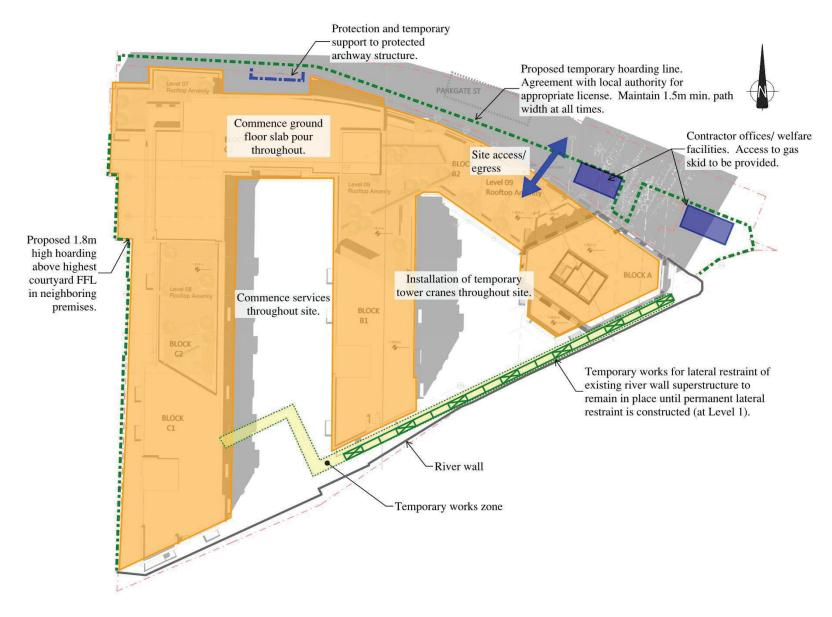
Figure 5 Overall sequencing of Works (5 of 6)
