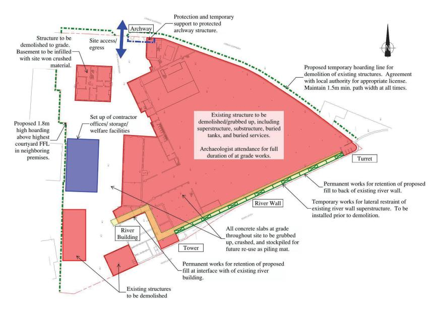
Figure 1: Overall sequencing of Works (1 of 6)
