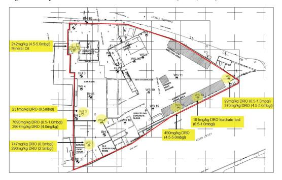
Figure 21: Hydrocarbon concentrations from the GI (IGSL, 2002)
