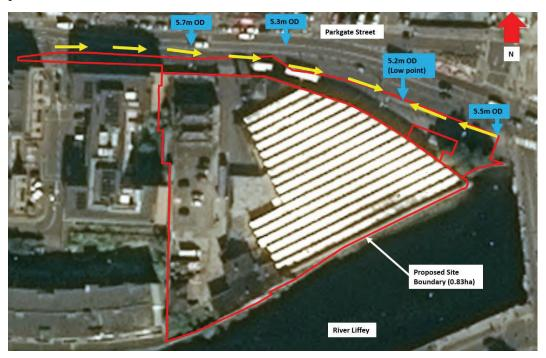
Figure 9: Surface water drainage directions (Source: adapted from Google Maps)
