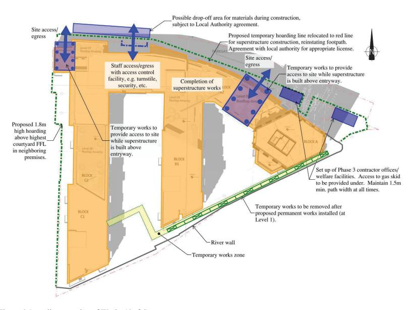
Figure 6 Overall sequencing of Works (6 of 6)
