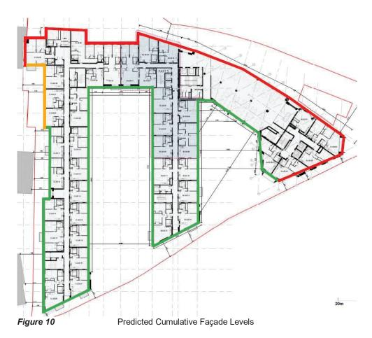
Taking into account the height of Block A1, a check of incident noise levels as the building increases with height has been done. At a height of approx. 32m incident noise levels decrease to a level where standard glazing is sufficient to ensure the required internal noise levels. Therefore glazing to facades of Block A1 from 8<sup>th</sup> Floor upwards are designated under the 'orange' and 'green' categories described above, i.e. these facades do not require upgraded glazing<sup>2</sup>.
